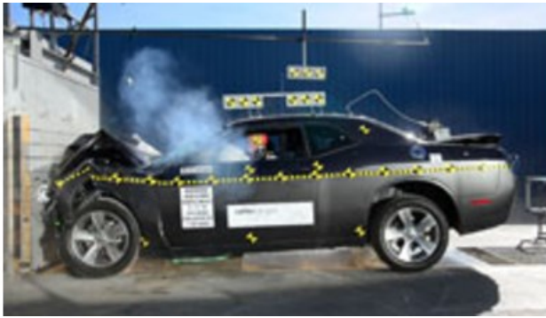
Fig. 1. Full frontal impact test (NHTSA-USA, 2018)
